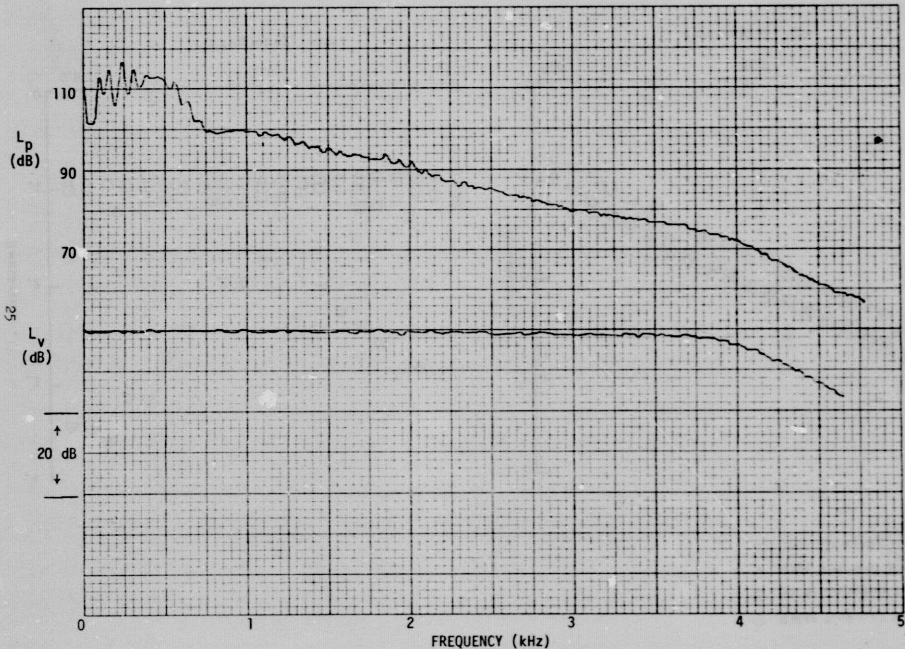
Figure 6. - Spectrum of sound pressure at face of sample (top) and spectrum of driver voltage (bottom).
