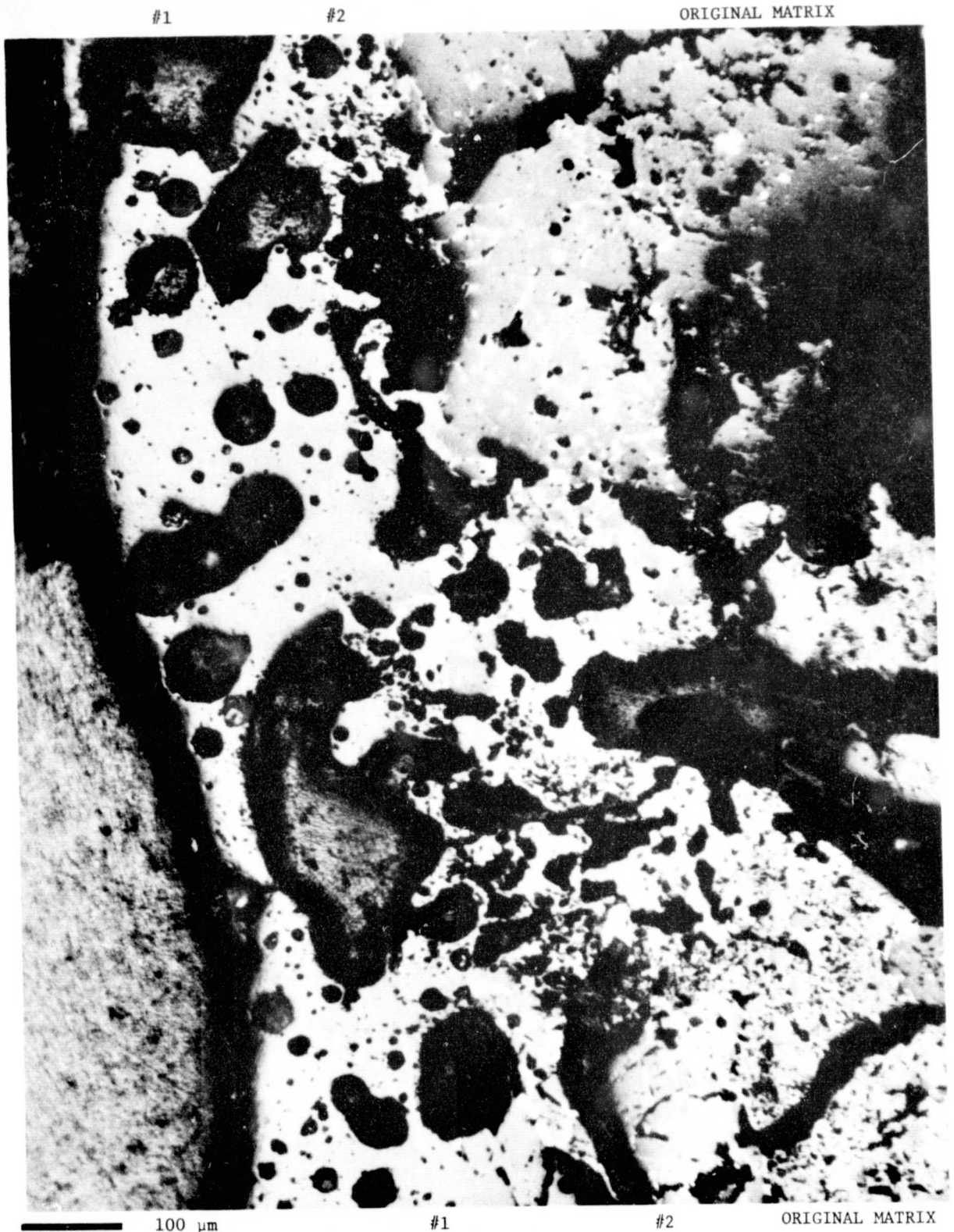
Fig. 2. Reflected light photomicrograph showing the outer (#1) and inner (#2) zones of the fusion crust of the Murchison meteorite. Bright grains in the inner zone are inclusions of iron sulfides invading the fractures and voids.
