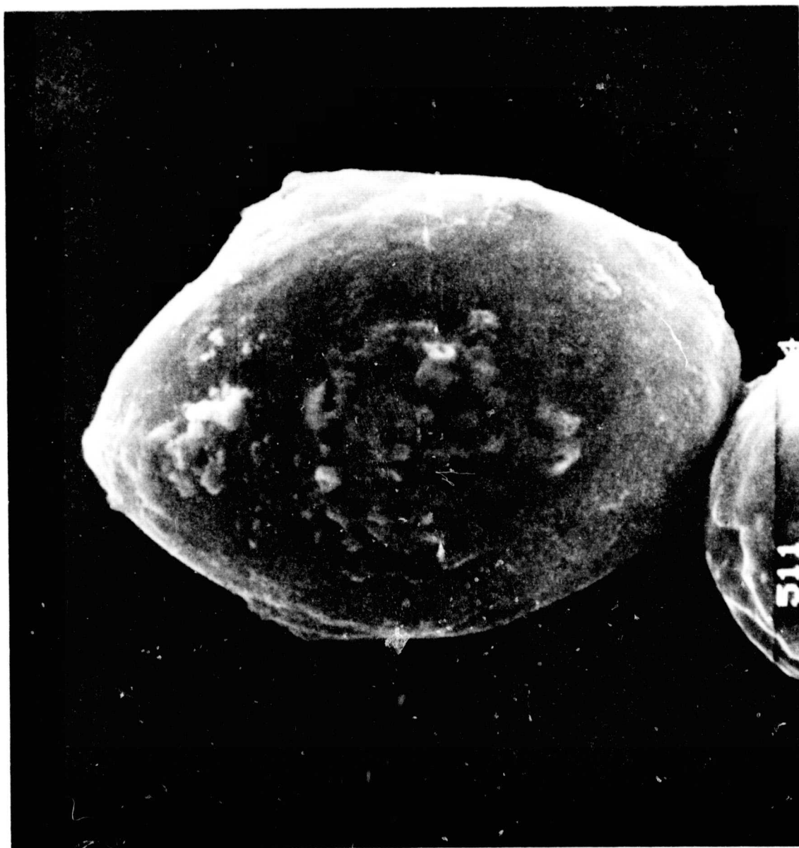
Fig. 6. SEM images of spherules ablated from the Murchison meteorite: (c) silicate spherule with an inclusion of the sulfide phase exposed at its surface.
