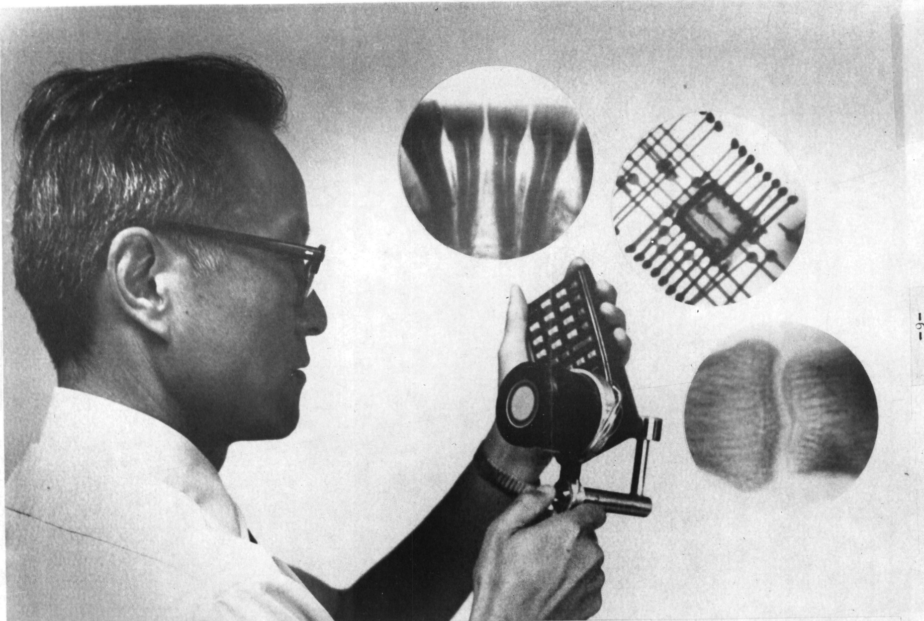
COMPACT X-RAY DEVICE -- Dr. Lo I Yin of NASA's Goddard Space Flight Center, Greenbelt, Md., examines a hand calculator with a demonstration model of his Lixiscope (Low Intensity X-ray Imaging Scope). Superimposed on the photo are images produced by the device. They include incisor teeth, integrated circuitry and the main joint of a forefinger.
