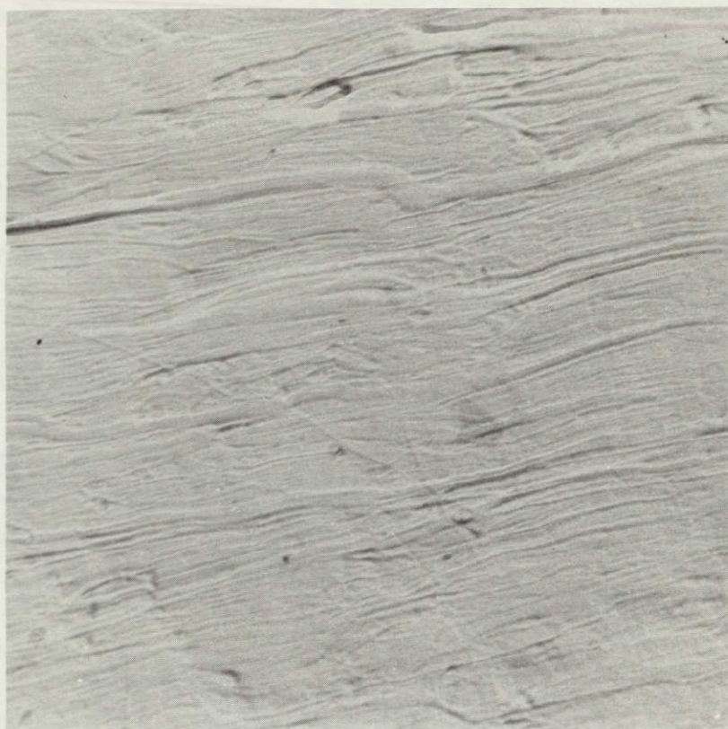
FIGURE 26. 30,000X TRANSMISSION ELECTRON PHOTOMICROGRAPH OF A TEFLON WEAR TRACK GENERATED AT 273 K
