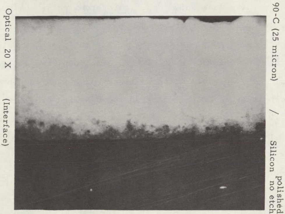
Figure 8. Silica/silicon interface at 20X for 25 \mu\text{m} crucible. The grey area at boundary is \text{SiO}_2 .
