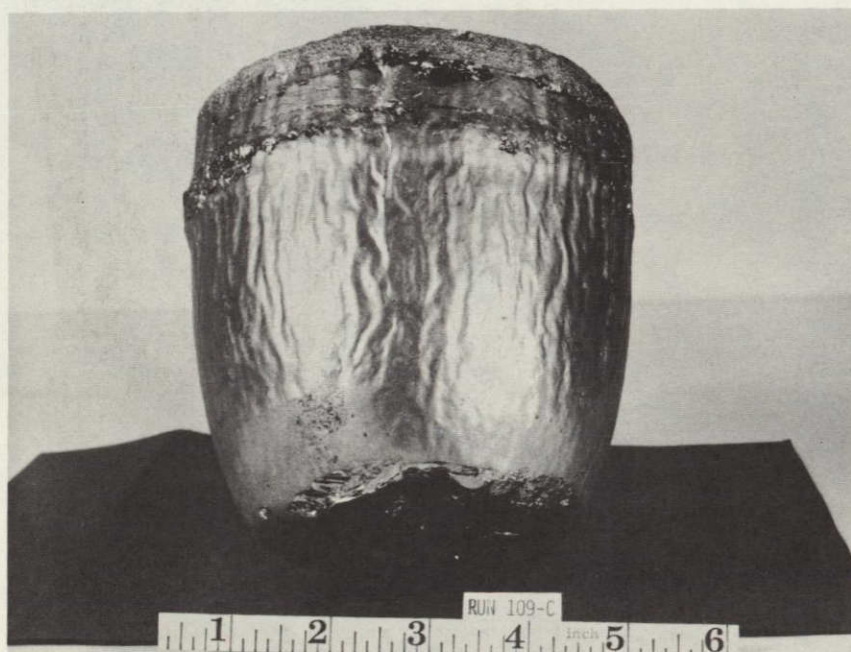
Figure 14. A crack-free 3.3 Kg silicon boule cast in run 109-C
