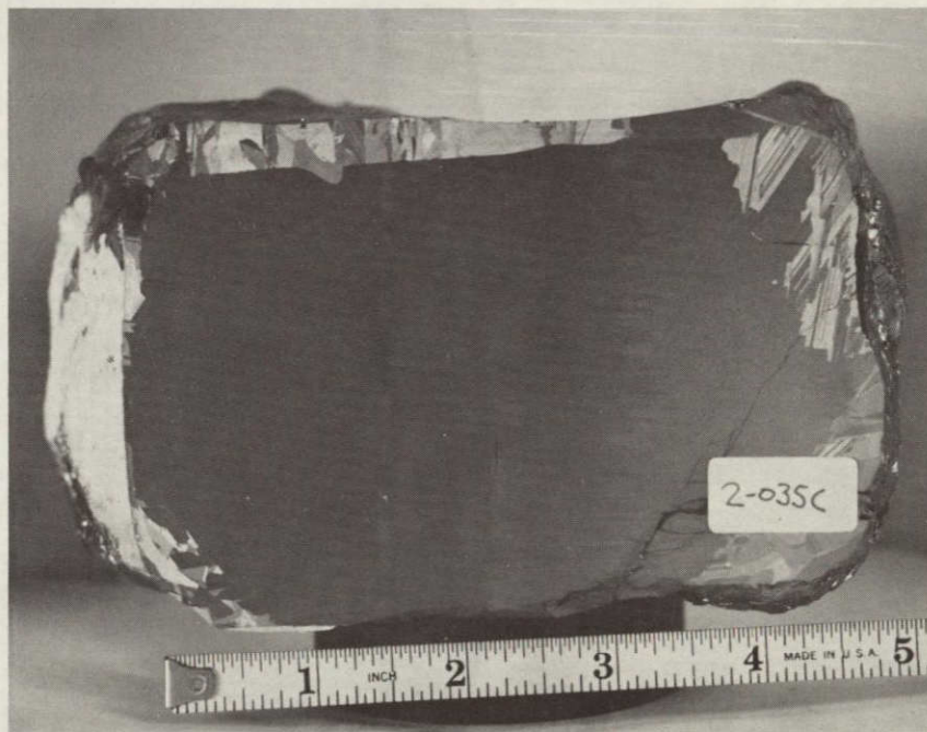
Figure 9. Polished and etched cross-sections of square ingots cast in run 2-034-C (above) and 2-035-C (below)
