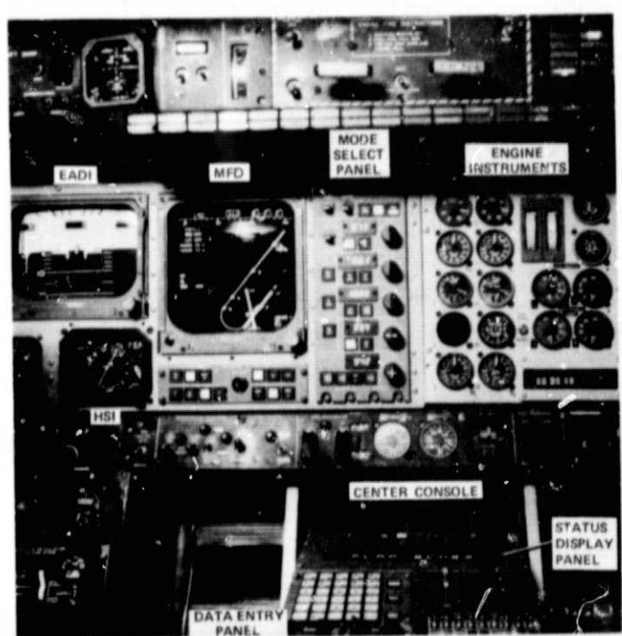
Fig. 9. Cockpit display installation.
