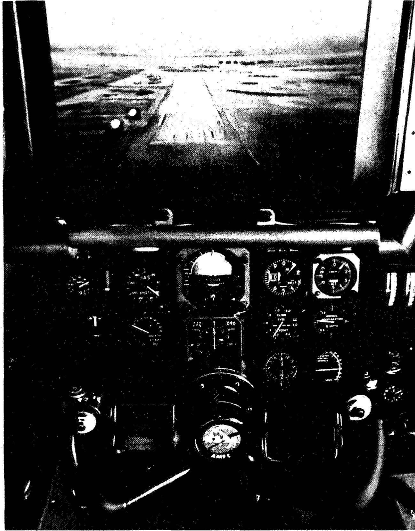
Figure 4. - Pilot's view from the cab of the Ames FSAA during the QSRA flight simulation.
