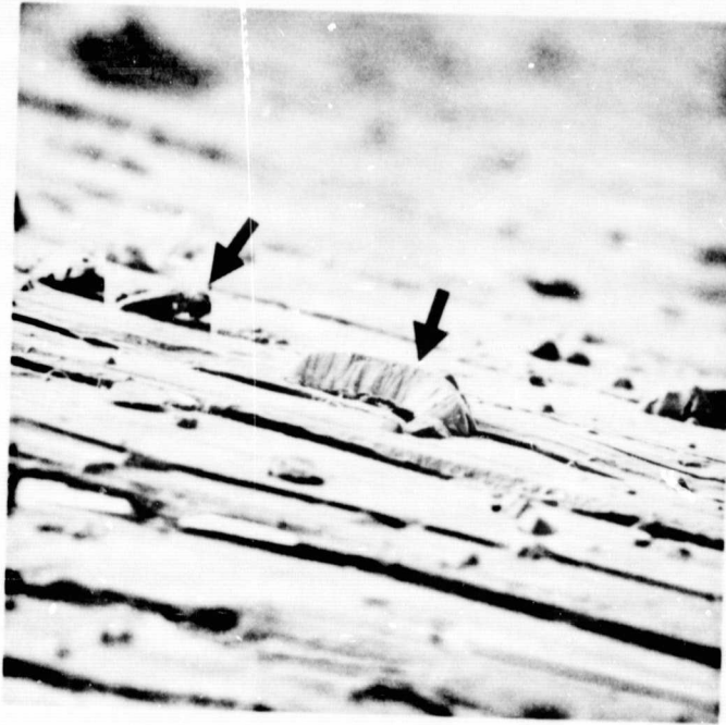
FIGURE 4. Surface of deposit of Figure 3, showing flake structure believed to correspond to powdery outer layer of deposit. Scanning electron micrograph. 350X
