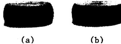
FIGURE 22. DEFORMED SAMPLES FROM NONUNIFORM COMPRESSION TESTS FOR DETERMINING WORKABILITY: (a) INCO 718 Specimen after 56 Percent Reduction, (b) AISI 1018 Steel Specimen after 70 Percent Reduction
