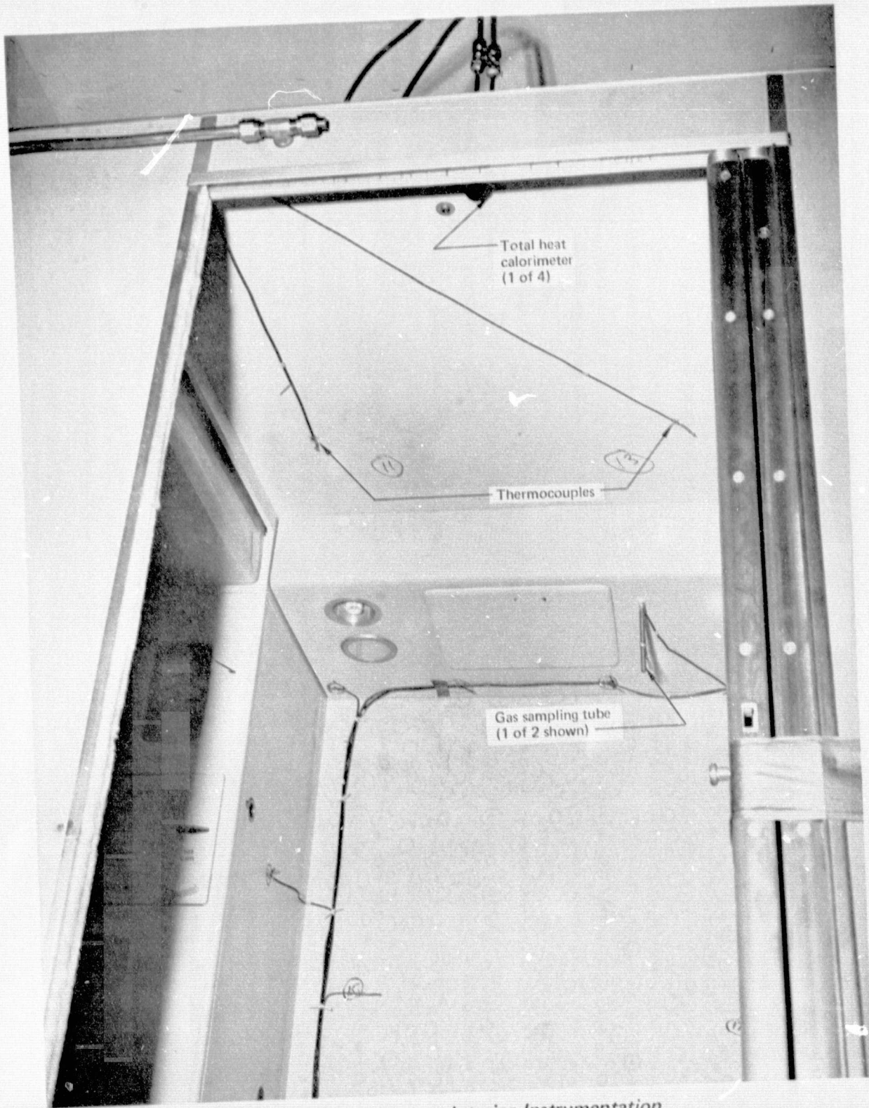
Figure 13.—Lavatory Interior Instrumentation
