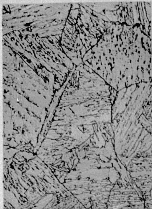
(b) Tempered & quenched at 500°C
