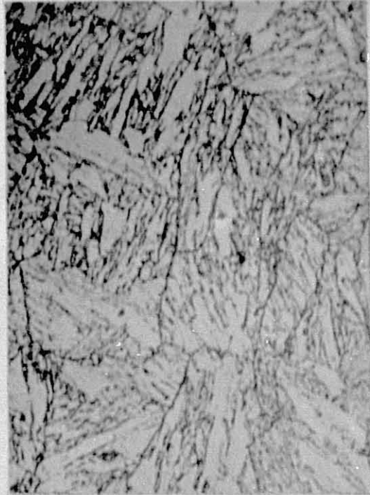
(b) Tempered & quenched at 550°C
