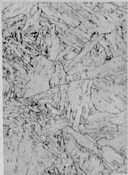
(b) Tempered & quenched at 550°C
