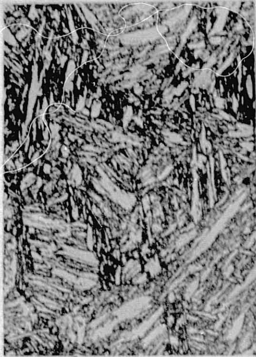
(b) Tempered & quenched at 550°C.
