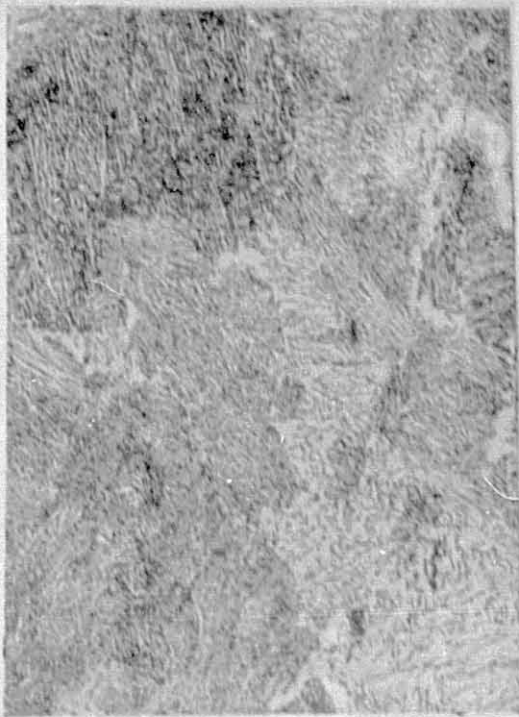
(c) Tempered & quenched at 685°C
