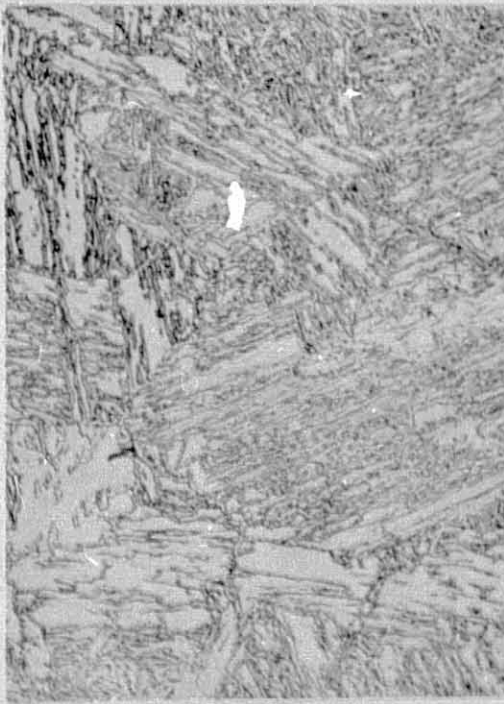
(c) Tempered & quenched at 600°C
