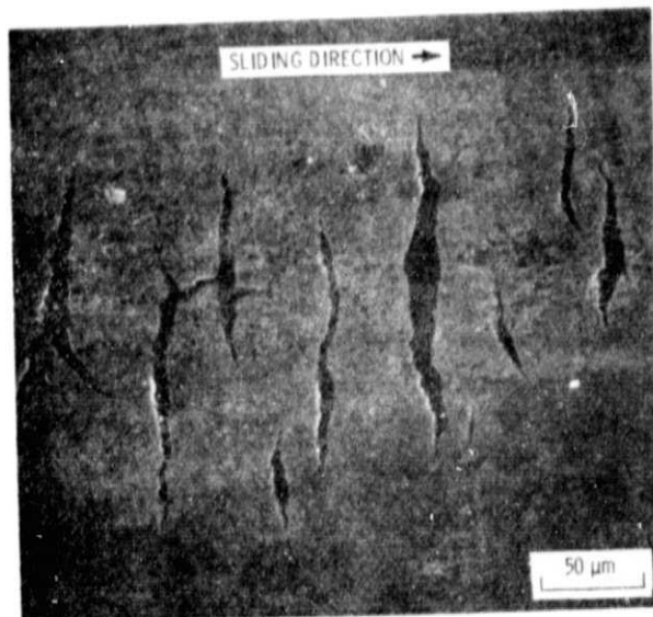
Fig. 9. - Thermal cracking observed on contact surface of 440C face seal seat.
