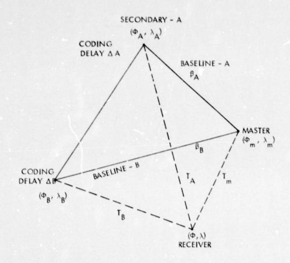
Figure 1. General Loran-C Configuration.
