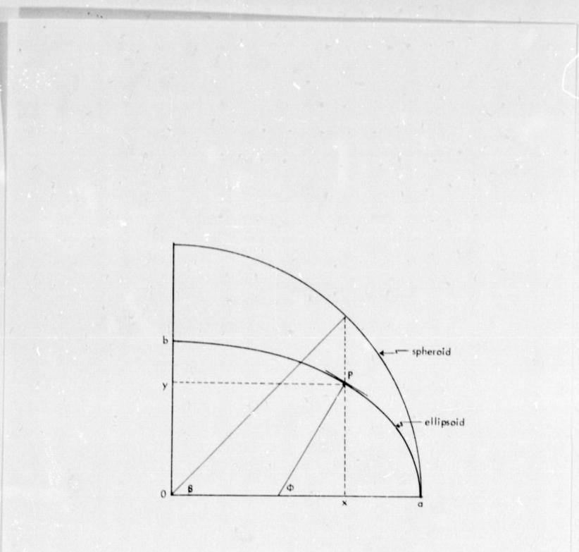
Figure 2. Relationship of Ellipsoid and Spheroid.
