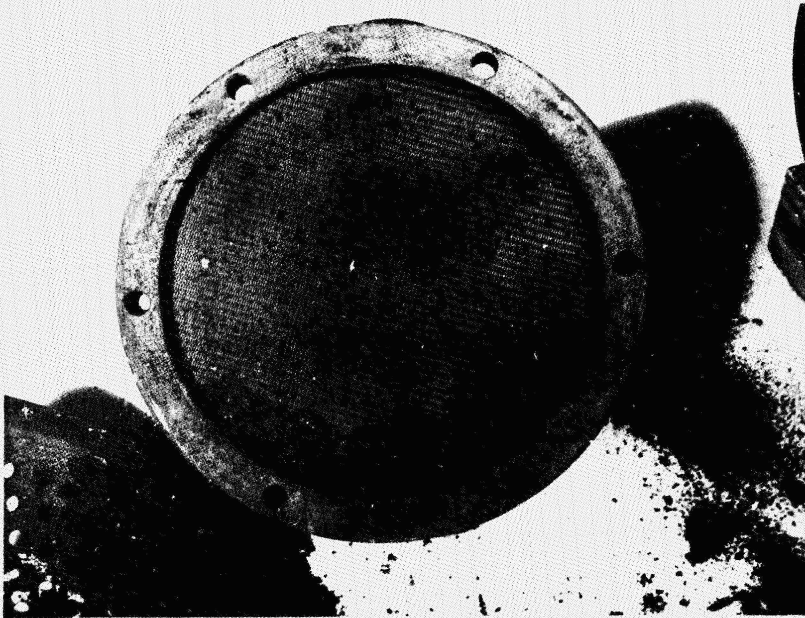
Figure 7. - Photograph of stainless steel screen removed from the settling chamber following decrease in facility performance.
