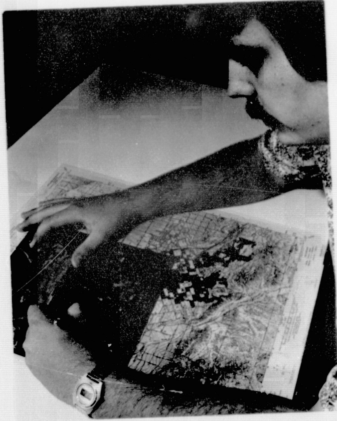
Figure 6: Manually transferring image data to the base work map (STEP 7a). One of the least expensive and most often used methods of transferring the data from an image to the base map is to inspect the photo, locate points on the photo and locate the corresponding points on the map and draw in boundaries between these points to outline the particular land use parcel on the work map. This method manually corrects or rectifies the distortions on the image created by the camera or other device used to produce the image. Likewise, any changes in scale from the image to the map can be made at this time. Visually changing scales is facilitated by using proportional dividers, 10 point proportional dividers are the most effective in this process.
