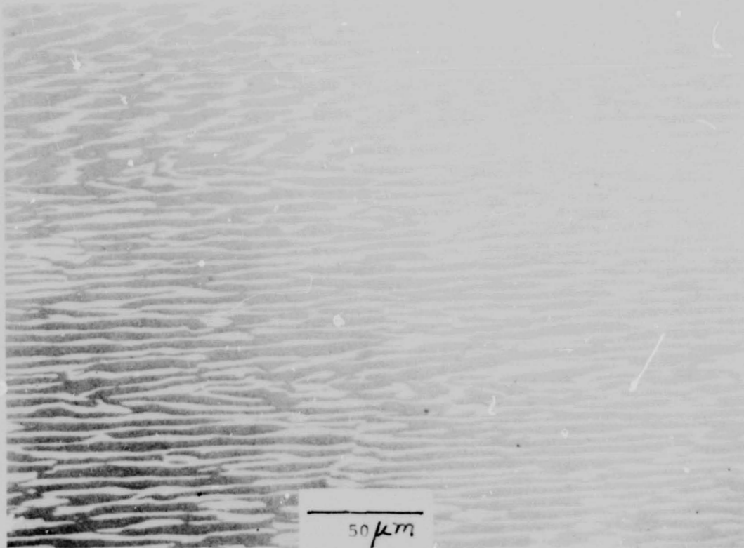
Figure 9-1. Longitudinal Section of the Fibrous Region in \alpha - \beta Alloy 32. R = 0.64 cm/hr
