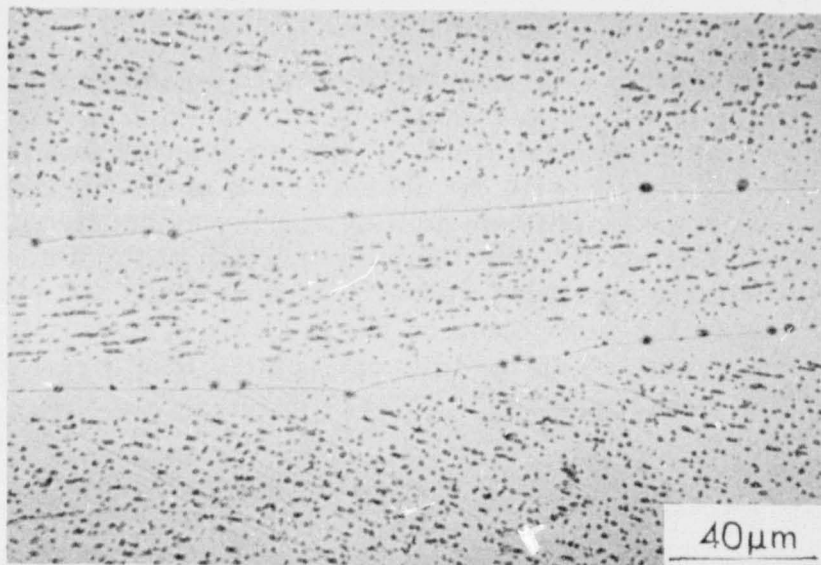
Figure 6-5. Longitudinal Microstructure of \gamma - \gamma' Alloy 20 After Thermal Cyclic Exposure to 1150^\circ\text{C} for 500 Hours
