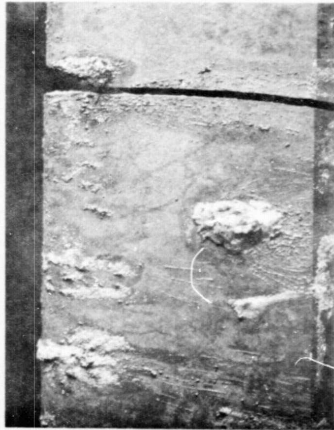
(b) Side view after failure during 126th cycles. Cooling.
