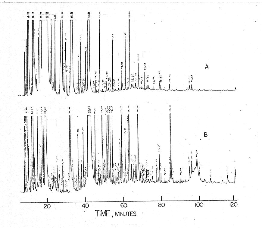
FIGURE 13. CHROMATOGRAM OF VOLATILE COMPOUNDS IN 100  $\mu l$  of hot coffee. Transevaporator used in the
