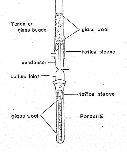
FIGURE 2. SCHEMATIC DIAGRAM OF A COMBINED HEADSPACE AND EXTRACTION SAMPLING PROCEDURE
