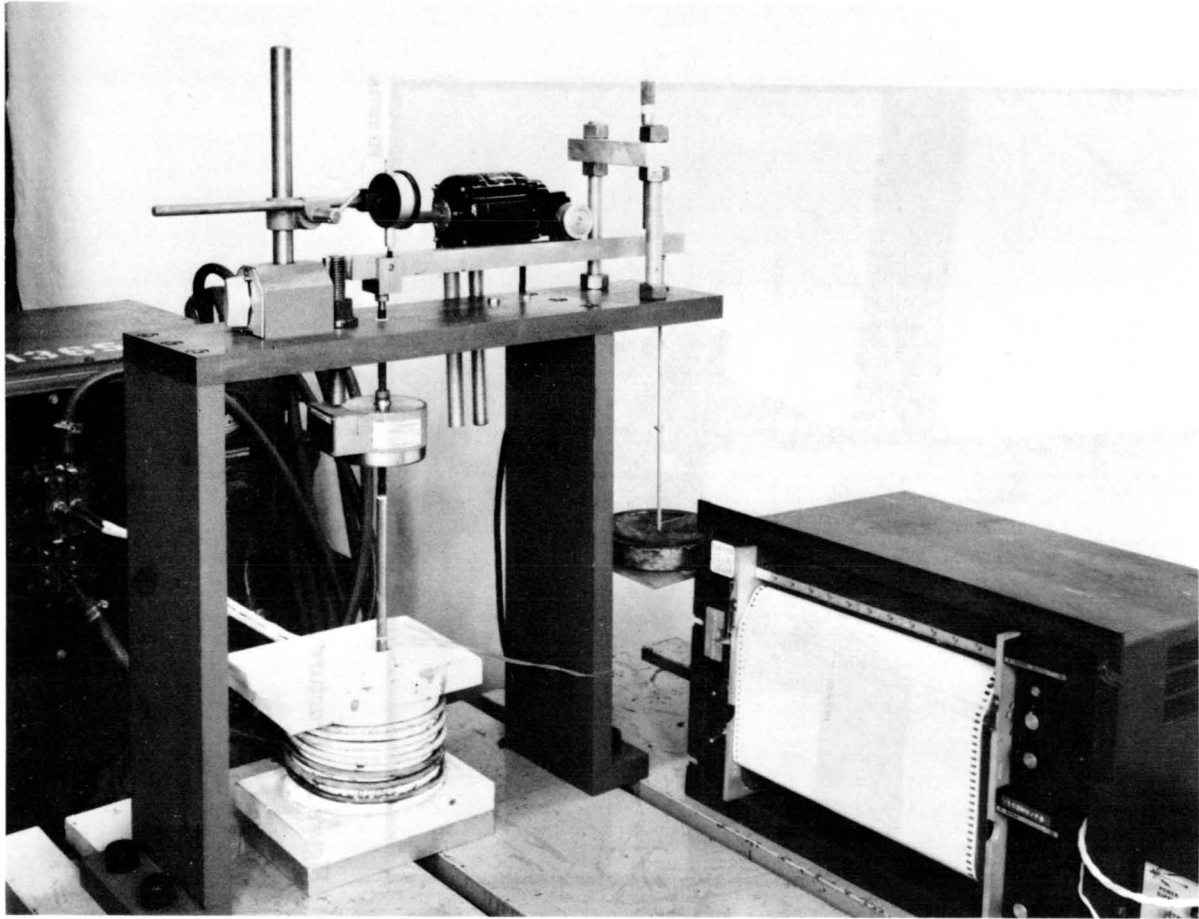
Figure 27. Fracture Mechanics Test Apparatus
