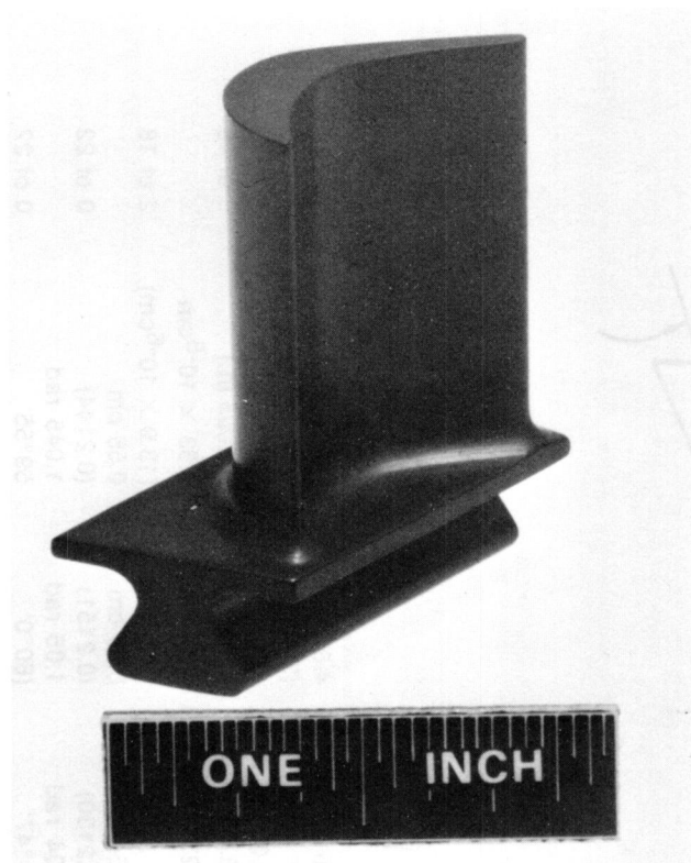
Figure 72. Finished Machined Ceramic Blade
