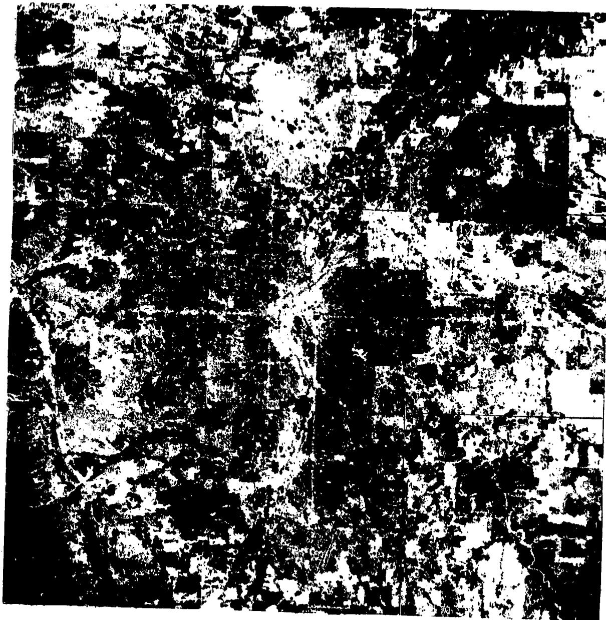
FIGURE 50. LANDSAT-1 MSS BAND 5 VISIBLE RED IMAGE OF THE DENVER METROPOLITAN AREA. Graymap of the August 15, 1973 image showing 676 by 676 image cells exactly as they were overlaid from the Landsat computer-compatible tapes to yield 1.111 acre per square cell. A square three-by-three array of these image cells of 10 acres exactly overlaid the square 10-acre cells of the landscape data planes.
