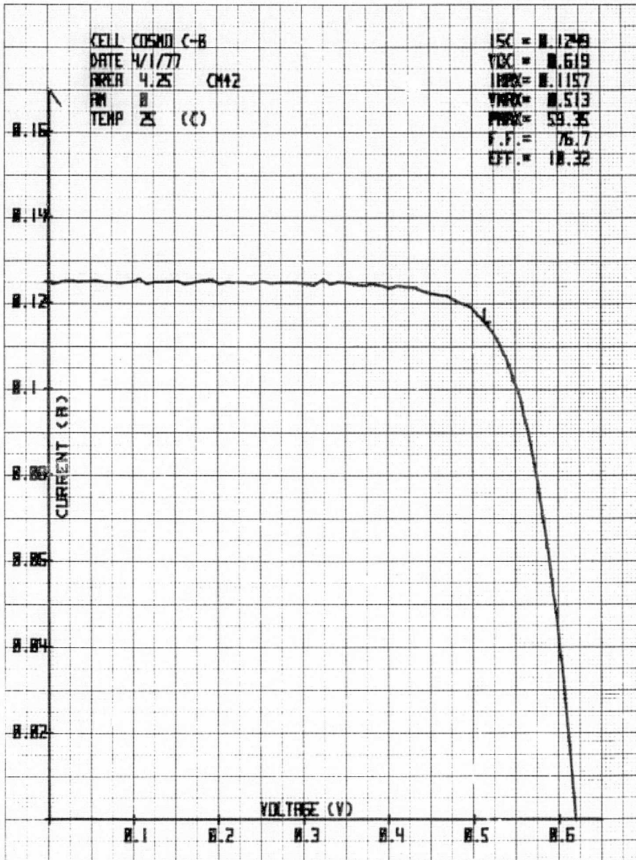
Figure D-5. Illuminated AM-0 responses and parameters measured at NASA-Lewis for sample C-B.
