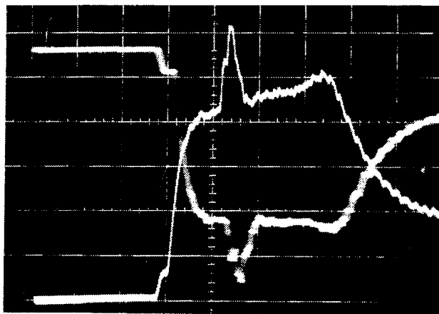
Fig. 25 Oscilloscope Record of Detonation Tube Stagnation Pressure with Burning Behind Reflected Shock and Overly Delayed Detonation
