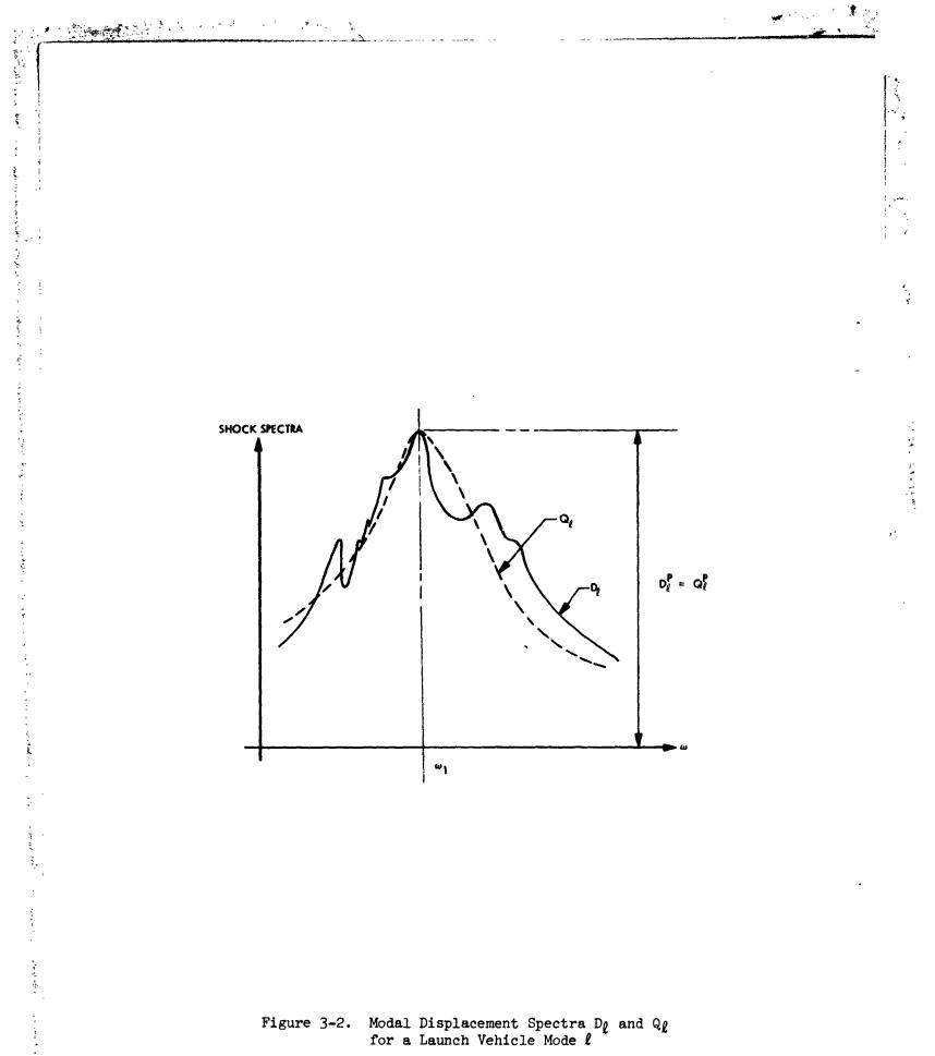
Figure 3-2. Modal Displacement Spectra  $D_{\ell}$  and  $Q_{\ell}$  for a Launch Vehicle Mode  $\ell$
