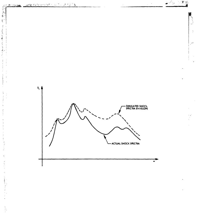
Figure 3-3. Shock Spectra Matching and Envelope
