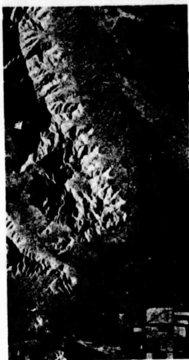
Figure 5. Aircraft Stereo Radar Image Pair, Opposite Side Geometry. X-Band, 12-km Altitude; Estrella Mountains, Arizona (Courtesy of Aeroservice, Goodyear)
