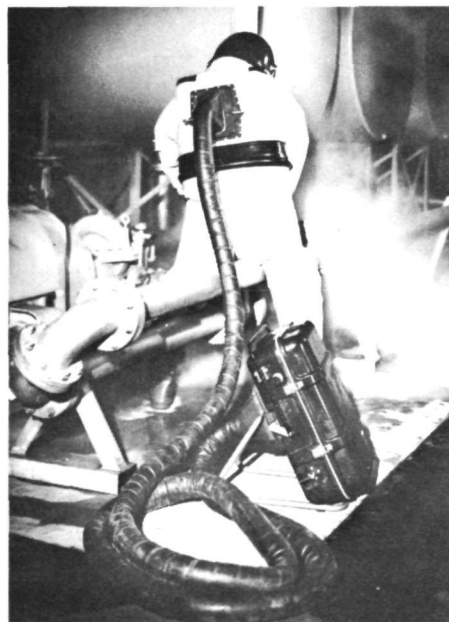
FIGURE A. LIQUID AIR PACK WITH UMBILICAL
