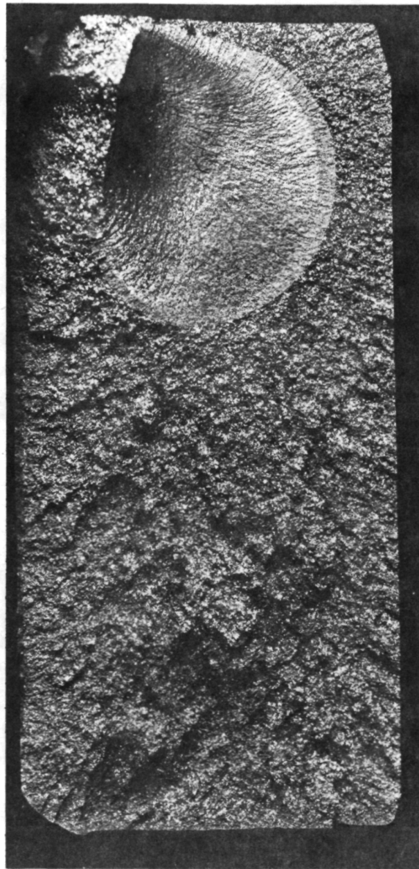
Figure 24. - Pitch-catch flaw map and fractograph of rail 5.
