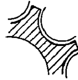
B) SALT CONTRACTION UPON FREEZING CAUSES A GAP TO FORM BETWEEN SALT AND CONTOUR SURFACE.
