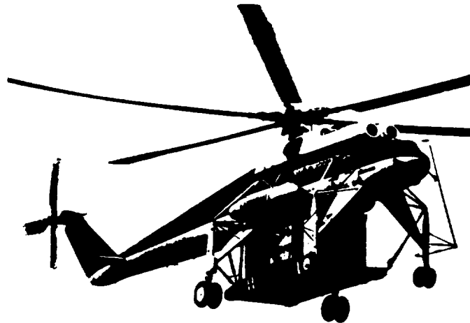
Figure 1.26 Large mechanically-driven, single-rotor helicopter (MIL MI-10 – W \approx 41\,000 \text{ kG} )
