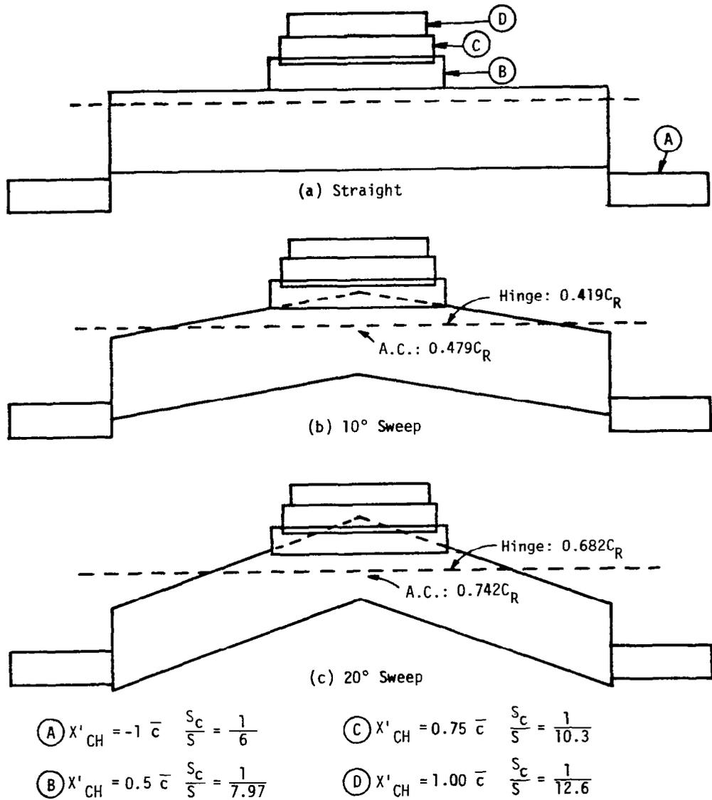
FIGURE 5. FREE-TRIMMER CONFIGURATIONS YIELDING THE SAME TRIMMED  $C_{LMAX}$
