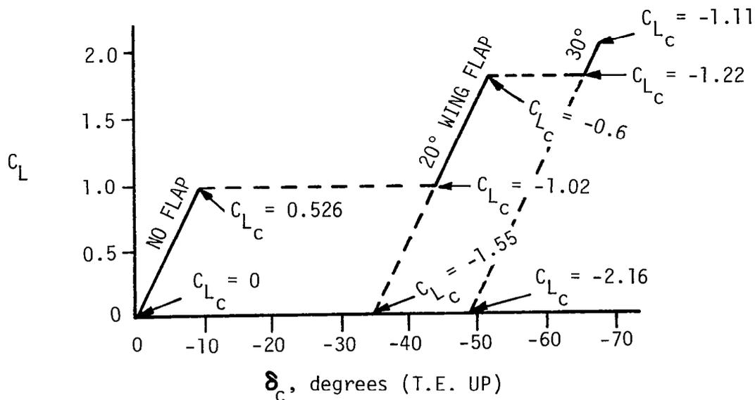
FIGURE 9. TRIM CHARACTERISTICS, STRAIGHT WING/AFT FIXED TRIMMER
