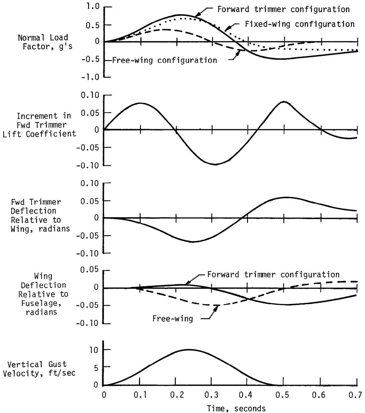
FIGURE 4. VERTICAL GUST RESPONSES ILLUSTRATING ADVERSE TRANSIENT EFFECT OF FORWARD TRIMMER
