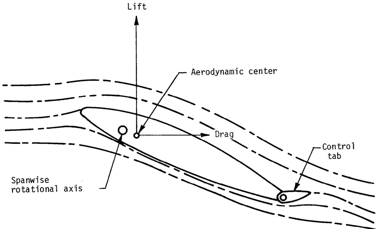
FIGURE 1. CROSS-SECTIONAL ILLUSTRATION OF THE FREE WING
