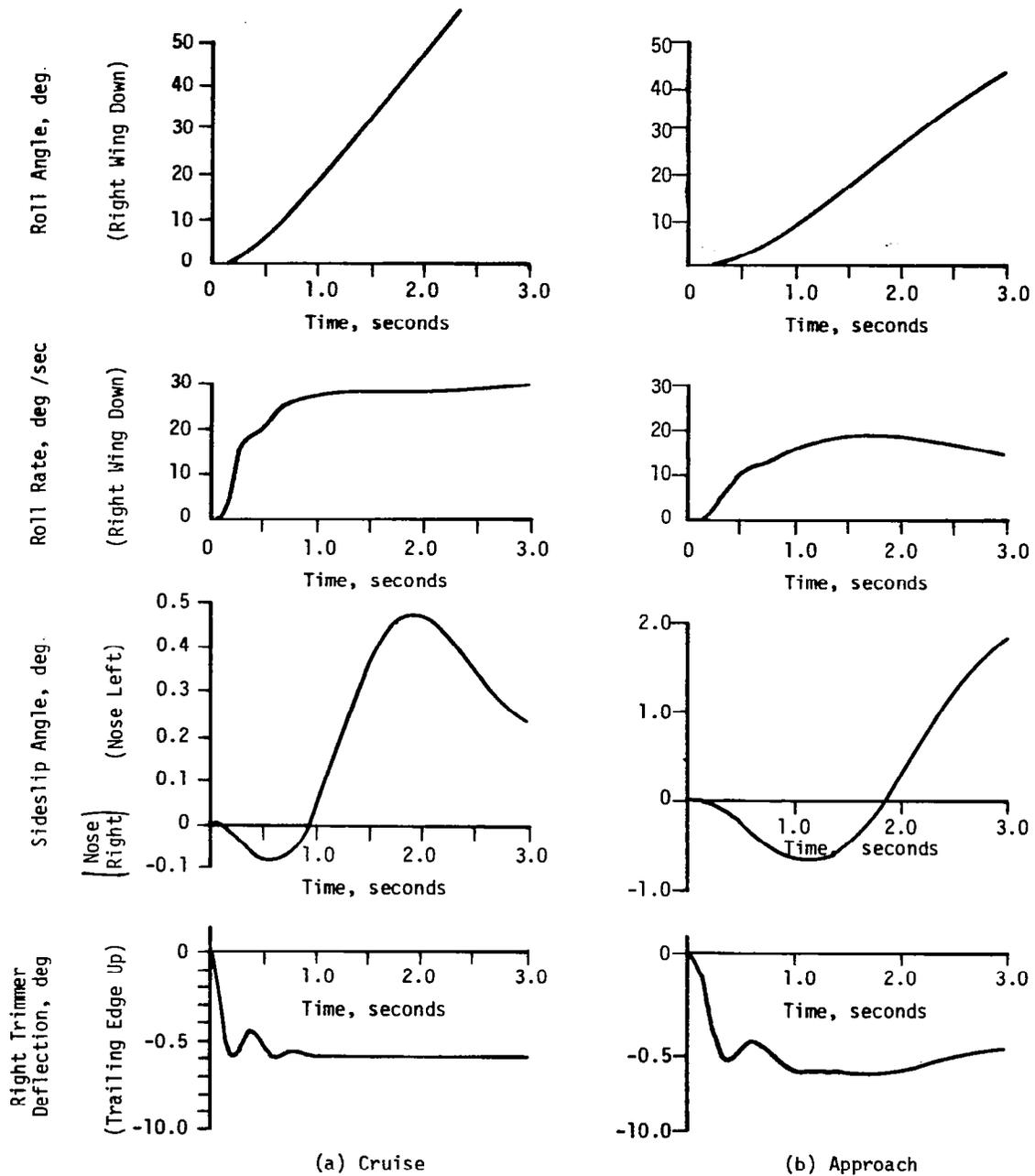
FIGURE 15. RESPONSES TO STEP LATERAL CONTROL INPUT, FREE TRIMMER CONFIGURATION
