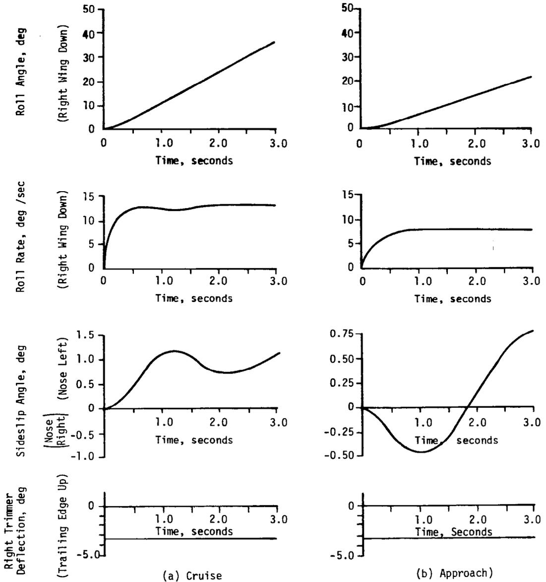
FIGURE 16. RESPONSES TO STEP LATERAL CONTROL INPUT, FIXED TRIMMER CONFIGURATION
