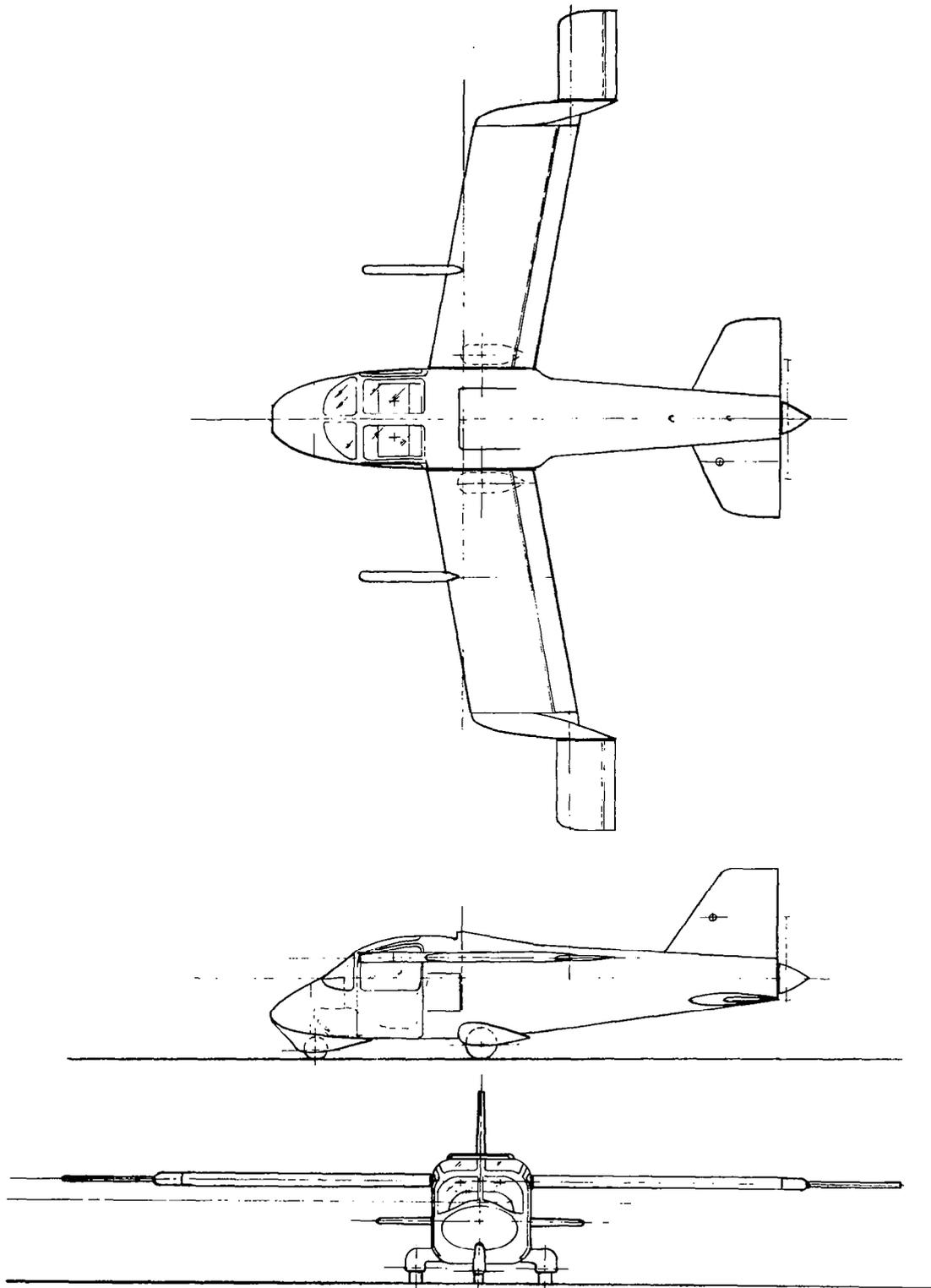
FIGURE 13. AFT TRIMMER CONFIGURATION WITH 10° SWEEP
