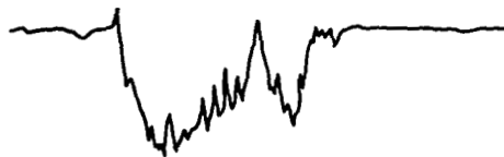
(b) Surface oxidized; average friction coefficient, 0.5.
