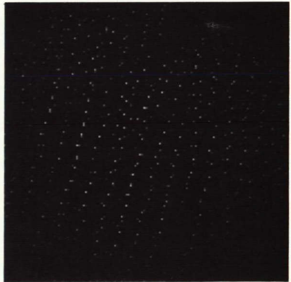
Figure 2.2(f) Histogram after decorrelation enhancement with Gaussian variance equalization.
