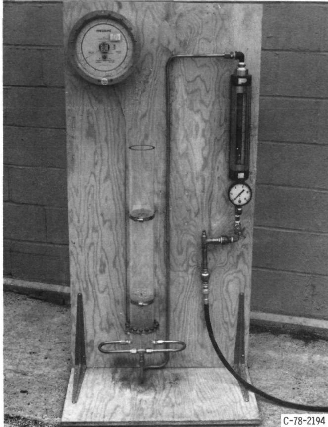
Figure 2. - Cylindrical cold-flow atmospheric fluidized bed used to measure particle density.
