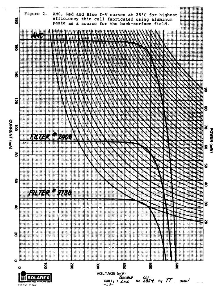
Future experiments will be concerned with investigating the effects of alloy time and temperature on the  $V_{OC}$  and maximum power. The goal is to produce  $V_{OC}$ 's consistently greater than 600 mV and  $P_{max}$ 's greater than 74 mW on 10  $\Omega$ -cm silicon.
