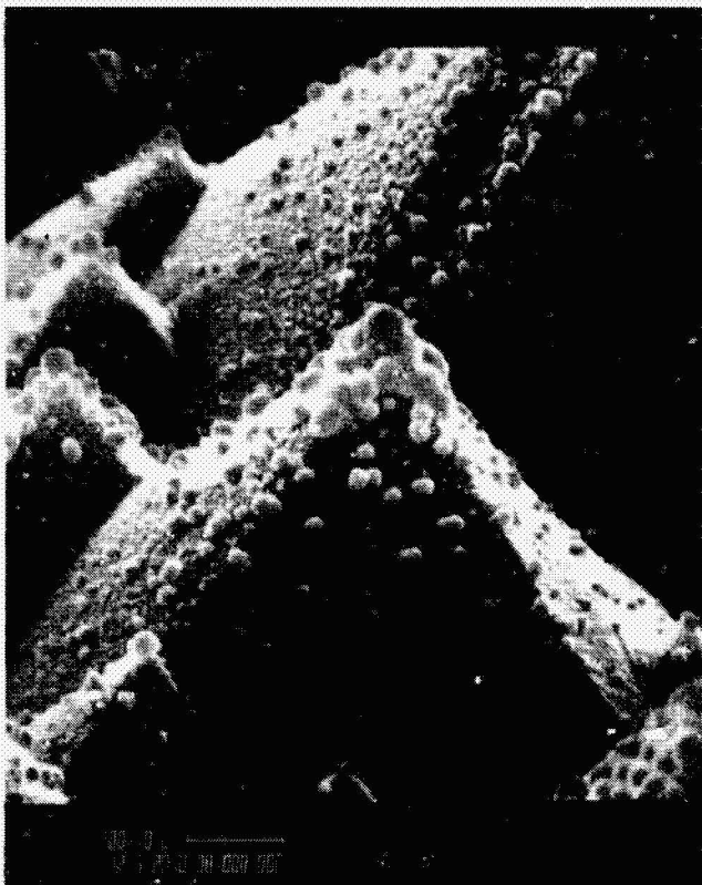
(a) N+ front textured surface showing large Pd grains on top of continuous, fine-grained Pd layer.
