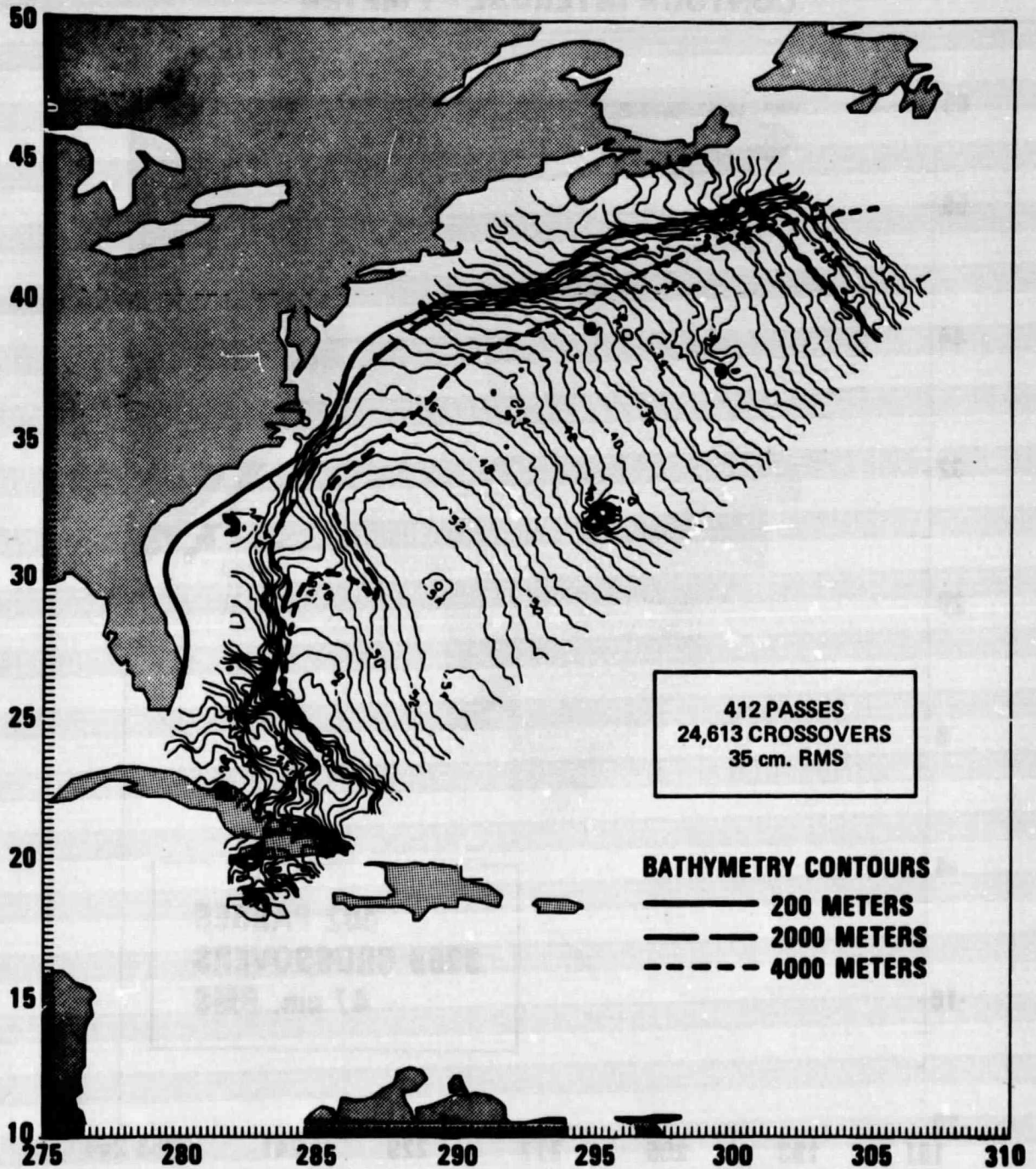
FIGURE 17. Contour Map of the Ocean Surface Derived from GEOS-3 Altimeter Crossover Data— Northwest Atlantic Ocean
