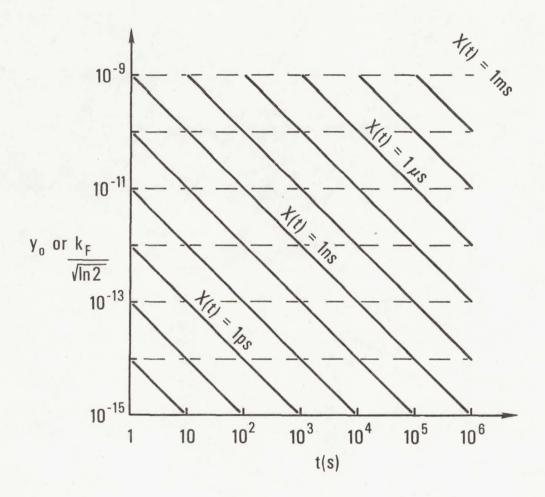
Figure 1. Largest allowable frequency offset,  $y_0$ , and flicker of frequency floor,  $k_F$ , as a function of time, t, after perfect synchronization. The achievable time accuracy, X(t), is the parameter.
