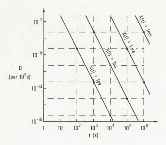
Figure 3. Largest allowable frequency drift coefficient, D, as a function of time, t, after perfect synchronization. The achievable time accuracy, X(t), is the parameter. D is used as a fractional frequency drift per  $10^5$  sec (approx. 1 day).
