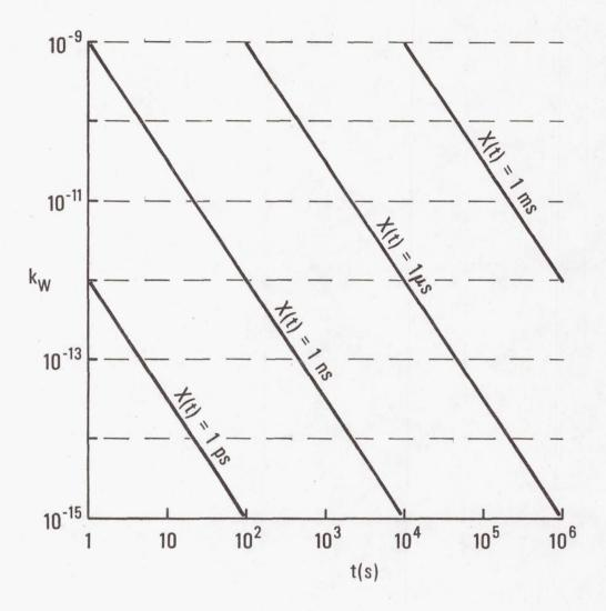
Figure 2. Largest allowable walk of frequency coefficient,  $k_W$ , as a function of time, t, after perfect synchronization. The achievable time accuracy, X(t), is the parameter.
