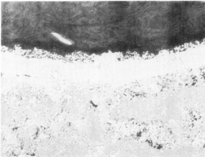
Figure 49. Ni-17Al Coating (No. 3) After Hot Corrosion Testing at 899°C
