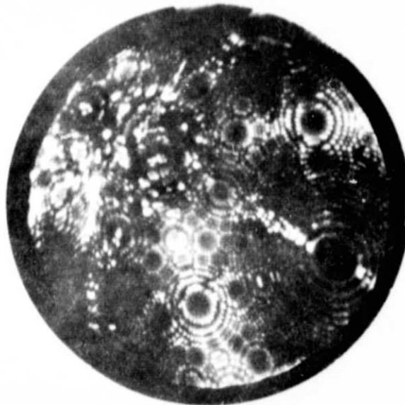
Figure 8. - Tungsten prior to contact (15,0 kV, helium image gas, liquid nitrogen cooling).
