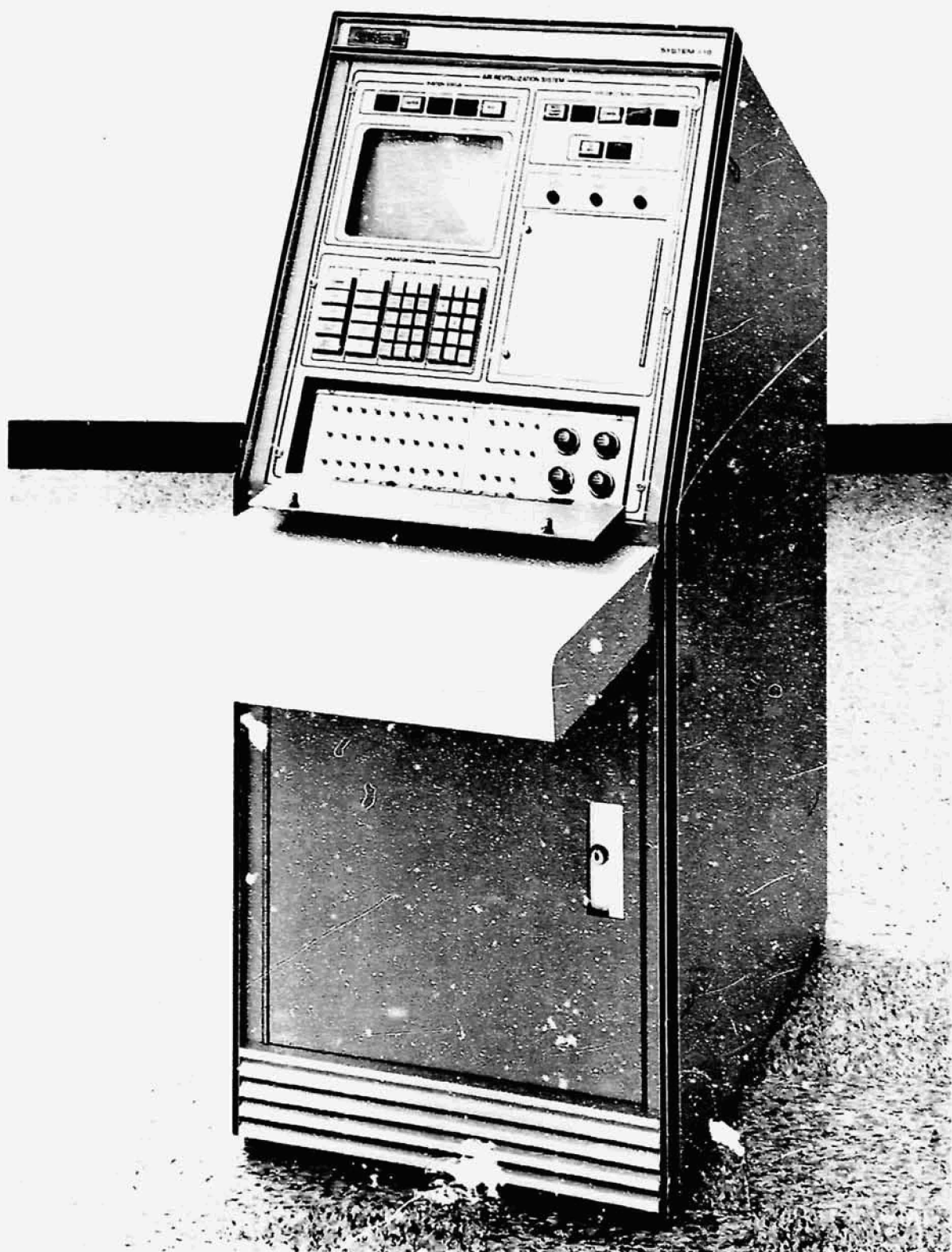
FIGURE 38 ARX-1 CONTROL AND MONITOR INSTRUMENTATION
