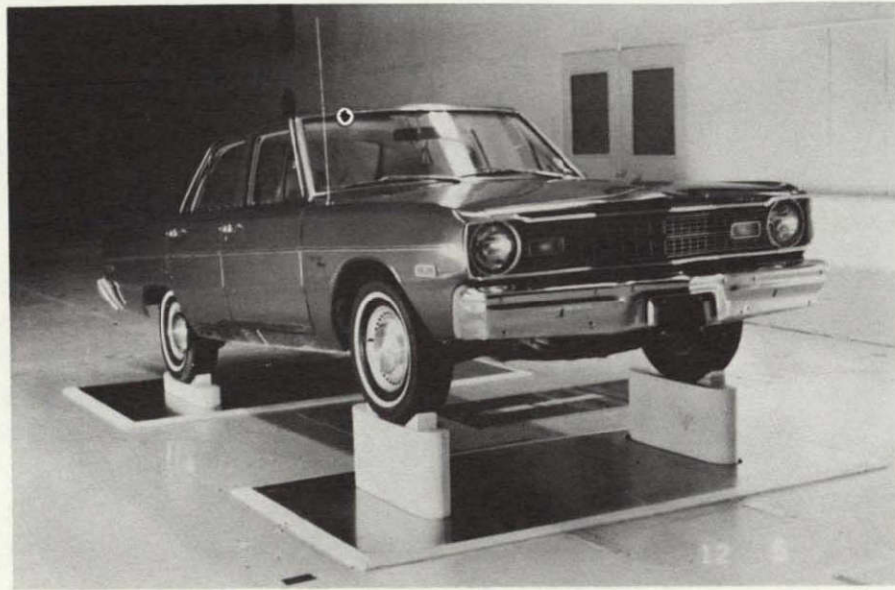
Fig. 3-14. Installation of 1974 Dodge Dart for ground plane tests at angle of attack in the 30 ft by 30 ft Wind Tunnel at National Research Council, Ottawa, Canada
