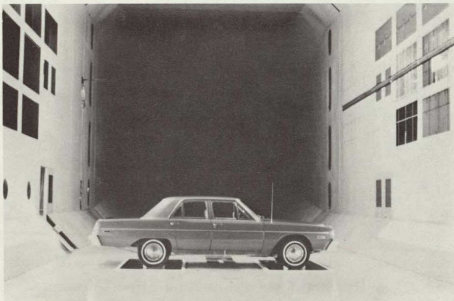
Fig. 3-13. Installation of 1974 Dodge Dart for ground plane tests in the 30 ft by 30 ft Wind Tunnel at National Research Council Ottawa, Canada
