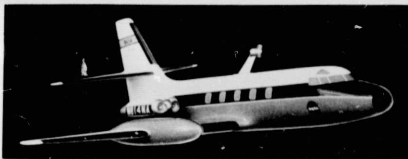
Figure 16. - Concept for high-speed propeller mounted on NASA Jet Star aircraft for in-flight acoustic tests.
