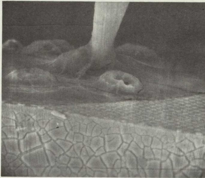
Figure 1. SEM Photograph of Dried Blood on 183 GHz Mixer Diode, 1150X
