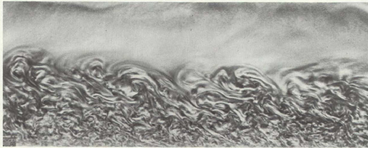
Figure 4. The structure of the turbulent boundary layer as visualized by the use of aluminum flakes in water; photograph courtesy of Brian Cantwell, Caltech (1978).
