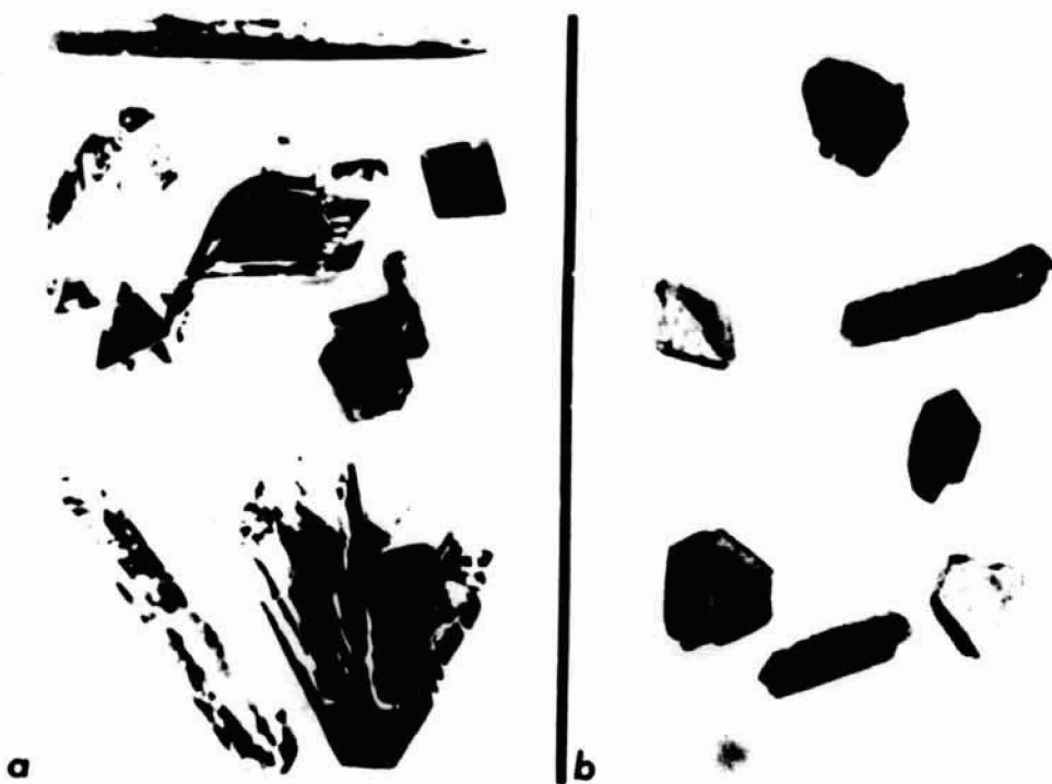
Figure 4-17. A comparison of GeTe crystals grown on Earth and in space. [Representative crystals grown by vapor deposition on Earth (a) are needles and platelets with distorted surfaces and hollow growth habits. The Skylab crystals (b) have considerably more compact habits and their facets exhibit a greater degree of smoothness and crystalline perfection. The dull appearance of the crystals grown in space results from condensation of the transport agent during the long cooling period dictated by the Skylab apparatus. In a dedicated process, this would be prevented by removing the ampoule from the furnace and quenching the vapor source.]
