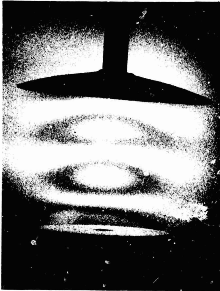
Figure 3-23. Reconstruction of a hologram showing the sound pressure field in a single-axis levitator. [A small sphere is levitated by the sound pressure at a null in the acoustic field. In one-g it is being supported by the high pressure region (dark area) below.]
