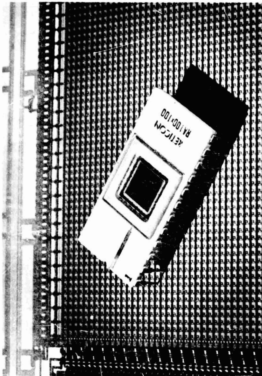
Figure 2-2. Reticon imaging array containing 10,000 discrete silicon photodiodes arranged with 60 micron center-to-center spacing. [For many applications as many as 10^6 - 10^7 detector elements are required, each with identical electrical characteristics. (Photograph courtesy of Reticon Corporation.) ]
