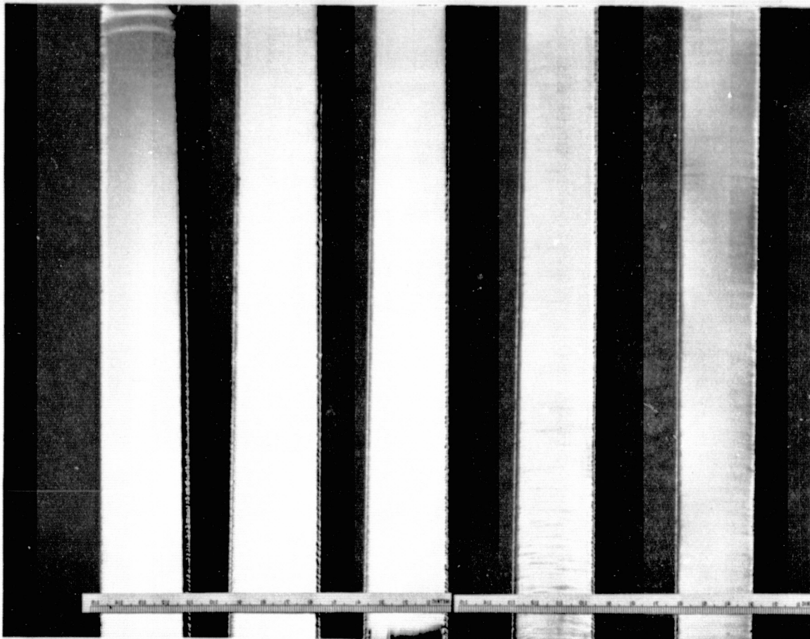
Figure 16 Close-up view illustrating smooth surfaces of as-grown web crystals. Faint striations are fine oxide particles deposited during growth.
