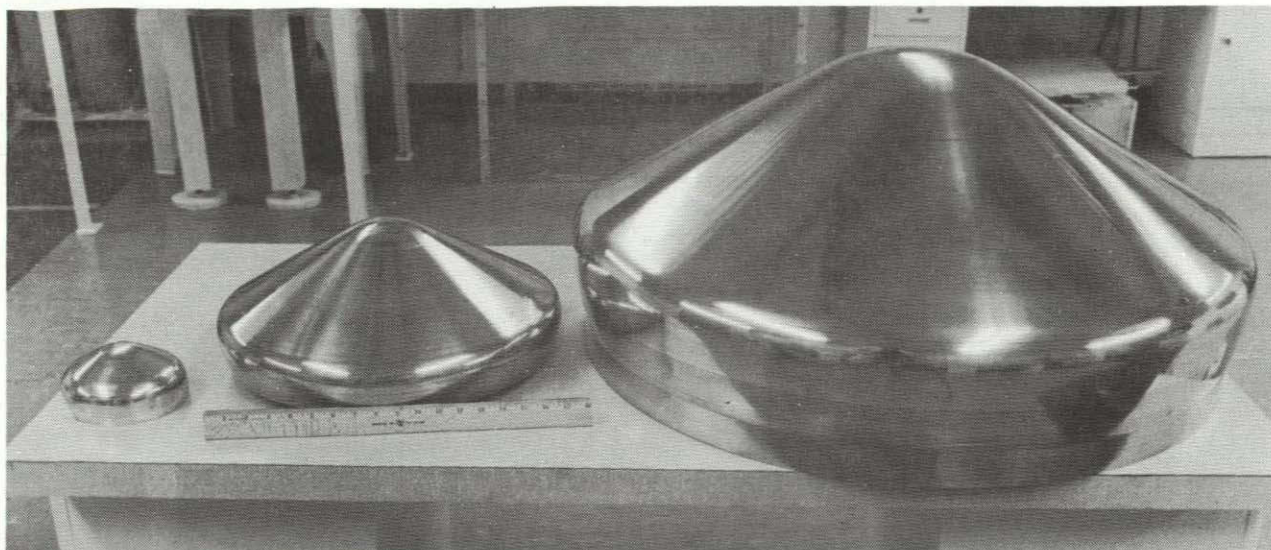
FIGURE 4.3-4 MASTER MODEL FOR 1/6 SCALE, 1/2 SCALE, AND FULL SCALE SILICA HEAT SHIELDS
