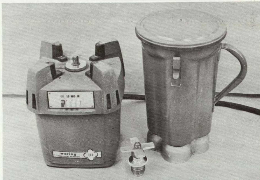
FIGURE 5.1-2 WARING BLENDER FOR WET CHOPPING HYPERPURE SILICA FIBERS
