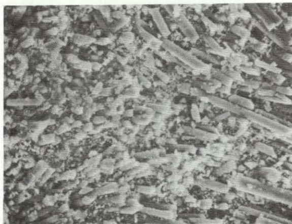
FIGURE 5.4-1 MICROSTRUCTURE OF A 100% SUPRASIL FIBER SLIP CAST SPECIMEN
