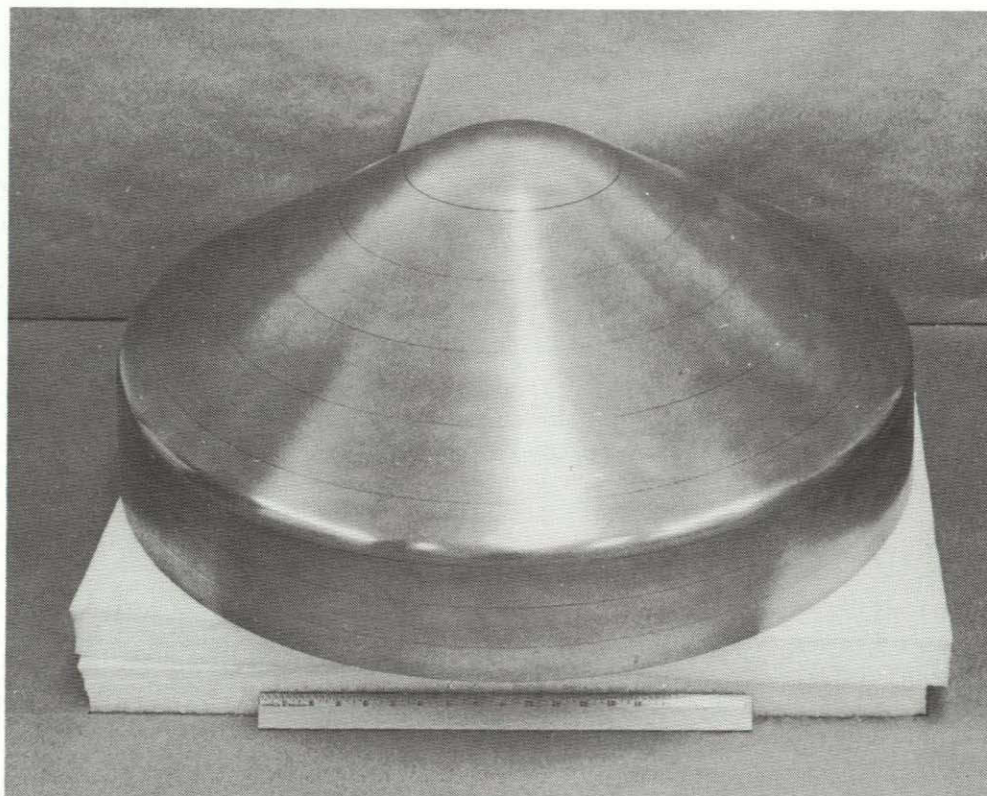
FIGURE 4.3-5 MALE MANDREL FOR FULL SCALE SILICA HEAT SHIELD
