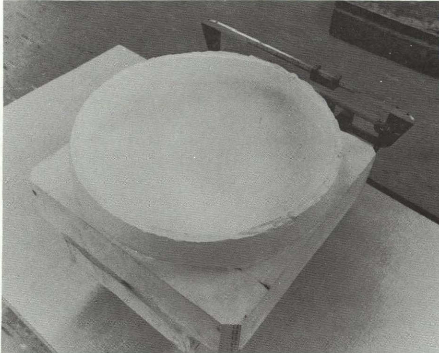
FIGURE 4.2-16 1/2 SCALE HEAT SHIELD NO. 3 AS REMOVED FROM CASTING MOLD
