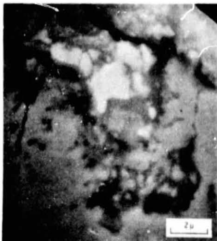
Figure 22. - Carbides imbedded in mixed oxides on IN-792 + Hf blade (R4).
