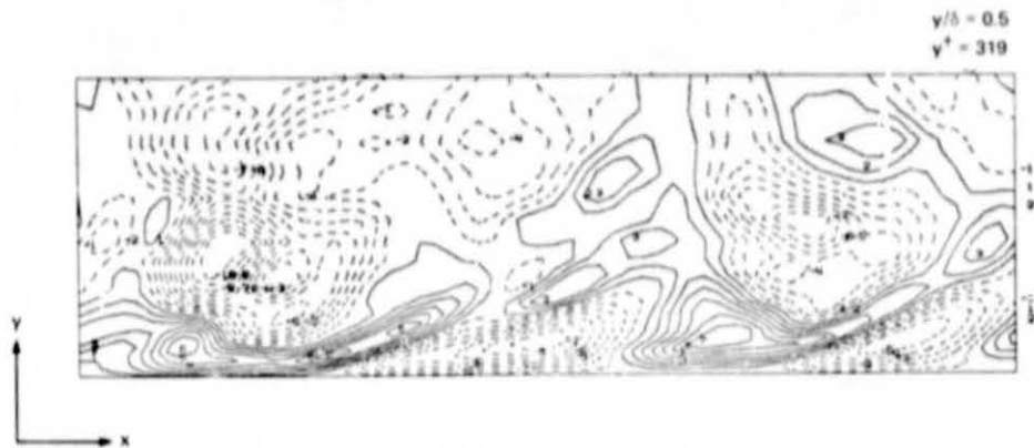
Fig. 7. Contours of \bar{u}'' in the x - y plane ( 0 < y/\delta < 0.5 ) at z = 15h_1 .
