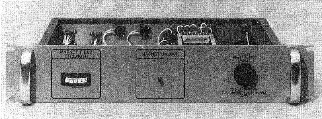
Fig. 5. Superconducting magnet control
